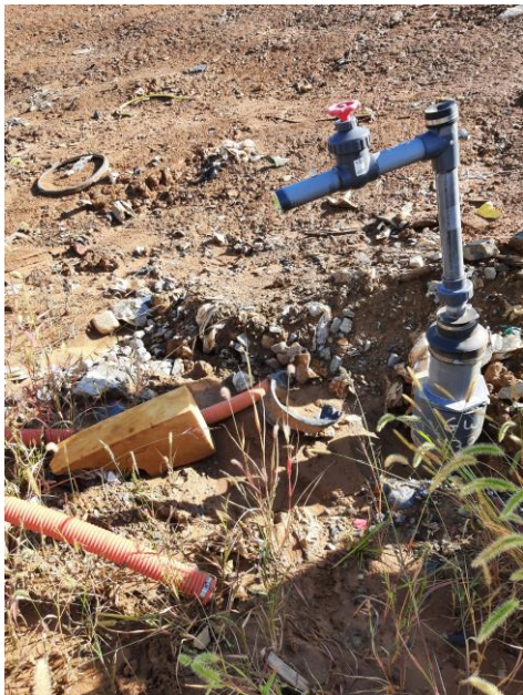
Photo 1: Disconnected hose at Gas Well GW-139.
