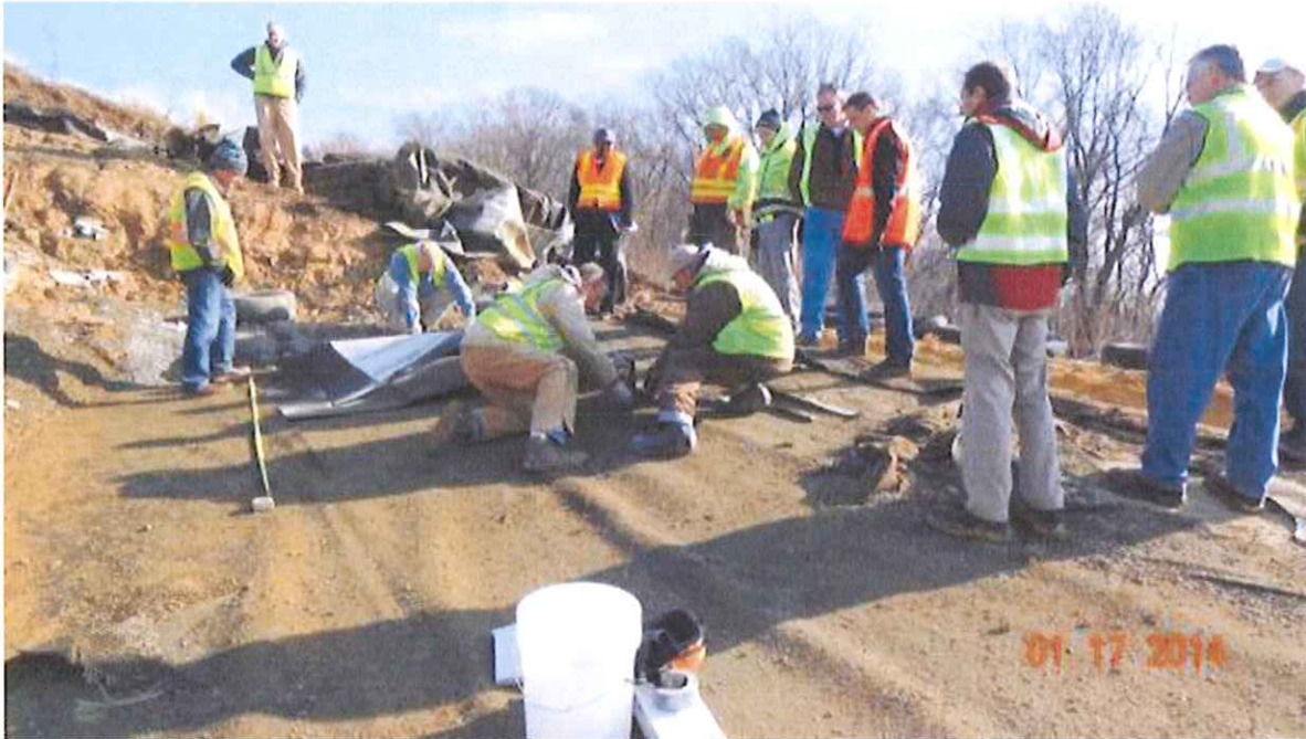
- Figure B-4 Obtaining South Liner System Samples
