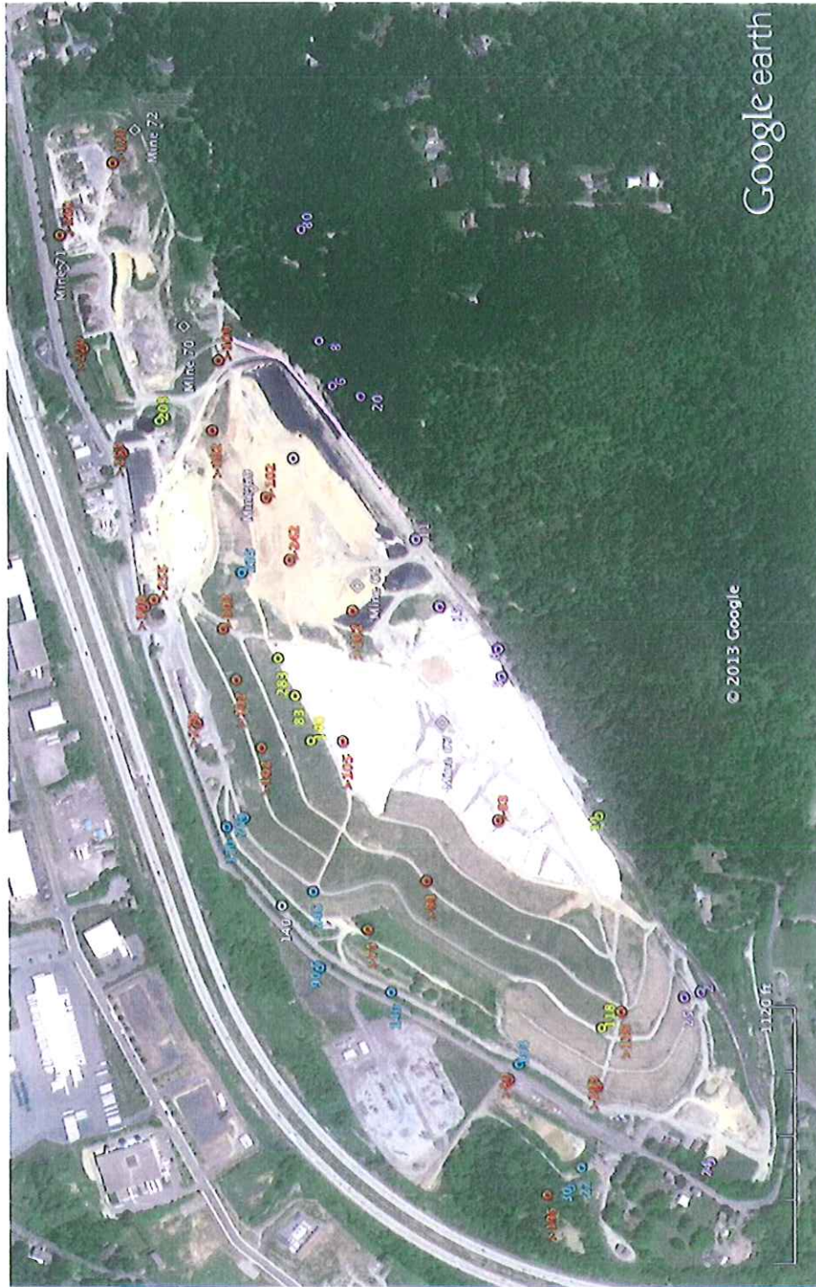
Figure 7. Depth to bedrock. Borehole locations are from previous geologic investigations at Chrin Brothers Landfill. Colors correspond to bedrock units identified in boring logs: Pink = Granite Gneiss bedrock; Yellow = Sandstone (Hardyston Quartzite); Blue = Leithsville Fm; Brown = Weathered bedrock (Saprolite); White = no geologic information on log. Mine locations (gray) were taken from Miller and others (1939).
